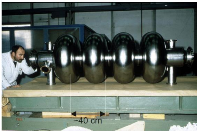
(a) Conventional rf cavity
