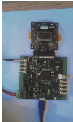
DAQ board (read-out) and Carrier card with ALPIDE chip
