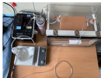
Figure 1. System of exhalation measurement.
