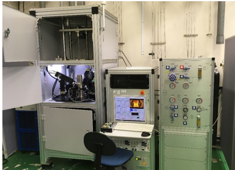
Figure 27: Optical furnace with 4 ellipsoidal mirrors (top left), prototype of a high pressure laser furnace with 3 lasers (bottom left) and the brick calibration cylinder (right).
