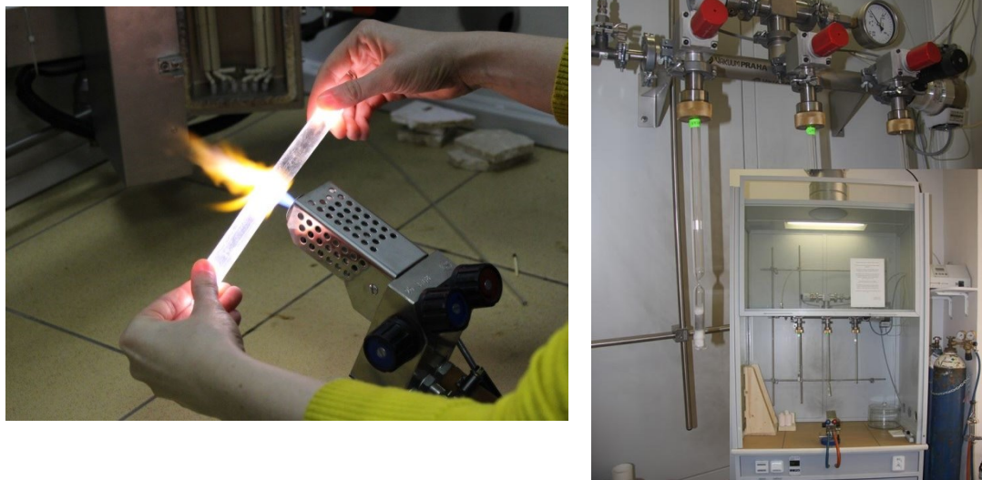
Figure 1: Making of the neck in quartz tube (left) and vacuum unit with glass sealing station (right) [2].
