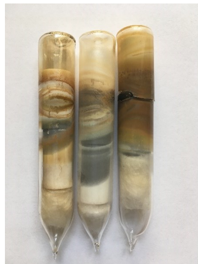
Figure 17: Temperature profile for growth of \text{Ce}_{3-x}\text{La}_x\text{Al}_{11} (left) and ampoules after growth process (right).
