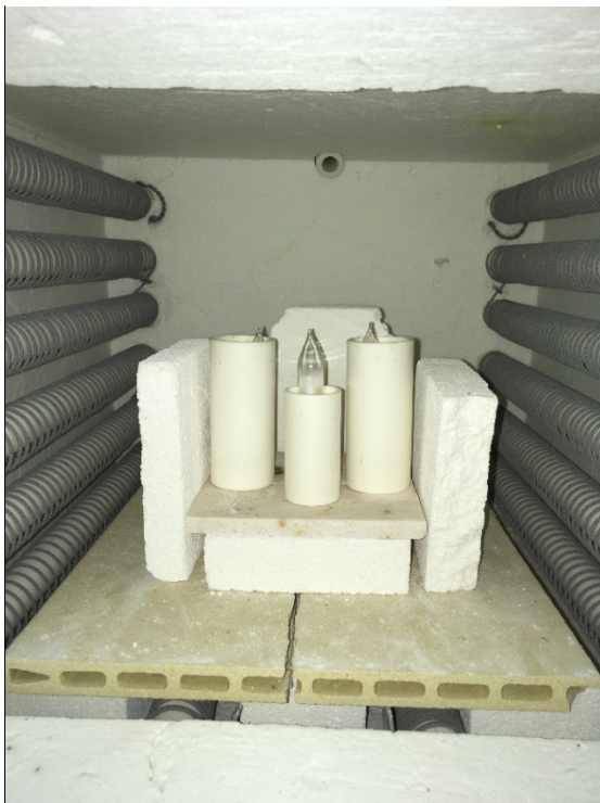
Figure 2: Furnace with ampoules in big alumina crucibles (left) and ampoules after decanting (right). The separated rest of the solvent element is visible in the upper tip of ampoules.
