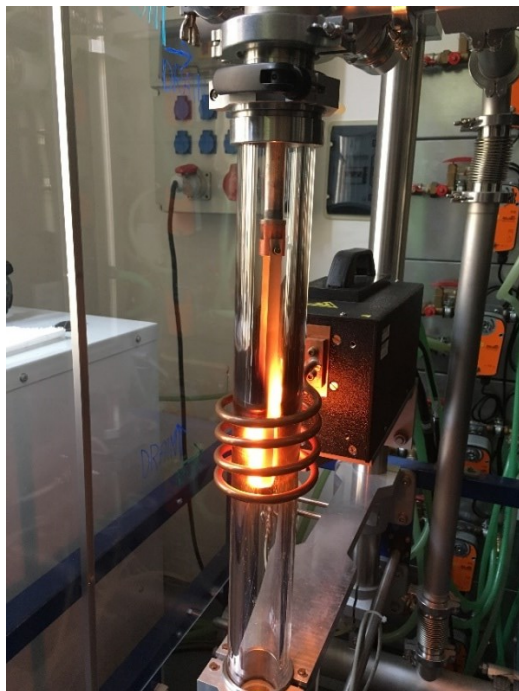
Figure 22: Heating up of induction furnace (left) and the opened Mo capsule with BN crucible (right). It is possible to see the scratch on the side of the BN crucible.
