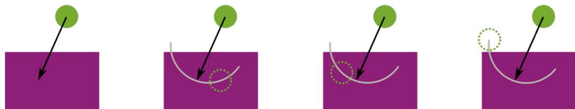
Figure 2: Operational phase: collision avoidance by course change - the blind velocity, searching for admissible positions, the final position.
