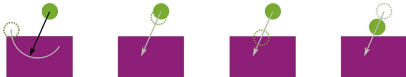
Figure 3: Operational phase: collision avoidance by slowing down - the course change does not work, searching for positions by shortening the blind distance, the final position.
