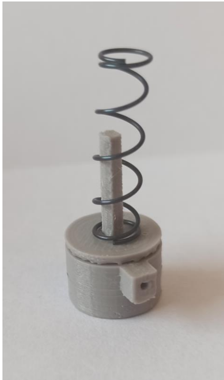
Printed ultrasonic transducer cup with the spring
