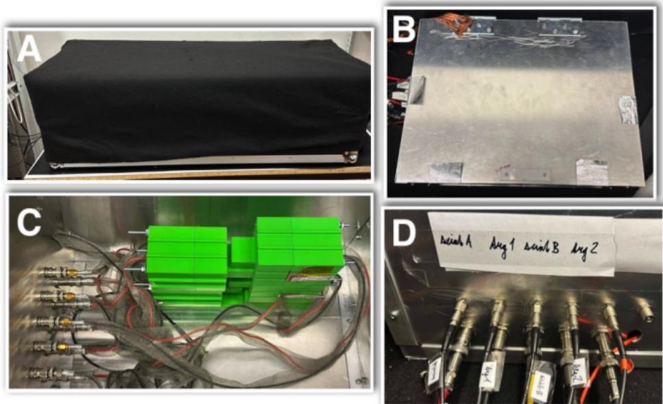
**Figure:** Set-up for sample characterisation using cosmic-ray muons: A) dark box, B) aluminium box, C) samples with PMTs, D) signal and HV patch panel.
