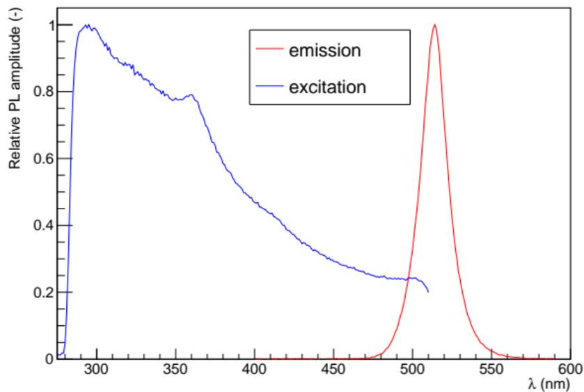
Figure: QD excitation (blue line) and emission (red line) spectra.
