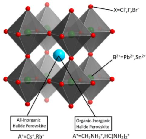
Figure: Diagram of metal halide perovskite  $ABX_3$ .
