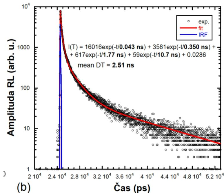
Figure: Time response of thin CsPbBr<sub>3</sub> layer on glass [3].
