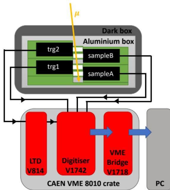
Figure: Set-up for sample characterisation using cosmic-ray muons.
