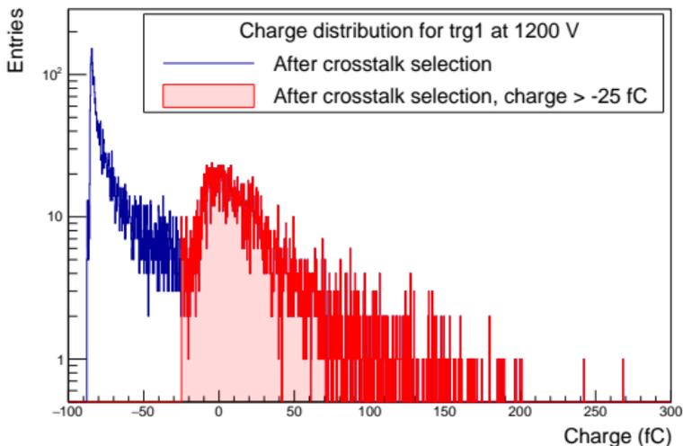
Figure: Charge distribution for BC-420 sample in module trg1 at 1200 V with charge selection.
