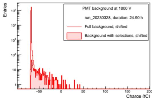
Figure: Background charge distribution: PMT without sample
