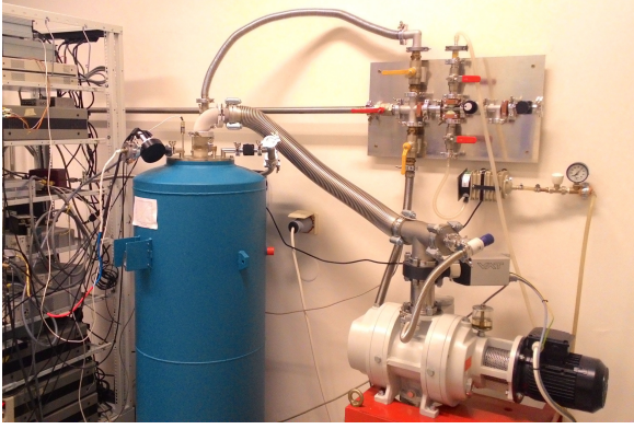
Figure 8: Photograph of the experimental setup - Left: cryostat, pipes where helium gas is flowing out of the system. Right: Roots-pump.
