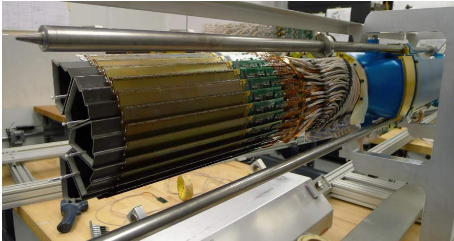
Figure 2.8: Structure of the Pixel detector. The sectors are grey and are carrying ladders with detectors, the readout cables are on the far side. Taken from Ref. [19].
